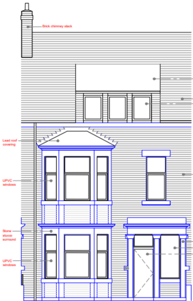
Existing Front Elevation
